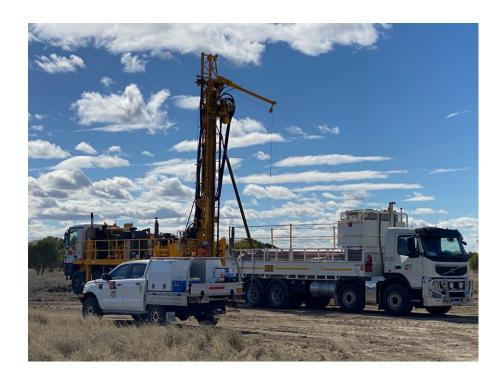
The drilling programme is expected to take approximately 10 days, providing core samples for analysis and allowing geophysical logging of the holes.
